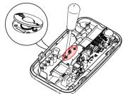
STEP 4 – Insert required Lens followed by Bezel and re-insert coloured screws and Lid
